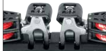
Toggles have a low pivot point to handle mainsheet loads up to 40 degrees from vertical, while allowing cars to roll freely.
