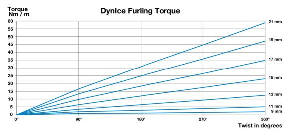
The torque is measured by twisting perpendicularly a length of 1000 mm and measuring the resistance in Nm. For example is the torque of 15 mm 23 Nm. As 1 N is equivalent to roundly 0,1 kg a 23 N is 2,3 kg. Imagine holding a stick which is 1 m long and on the end are the 2,3 kg hanging. That is the force needed to twist the DynIce Furling cable one full twist and that is quite high force.
