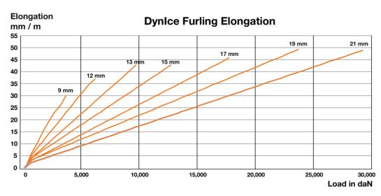
The elongation in mm for each diameter is similar as the top end of the line represents the full elongation of 1000 until it breaks. One m of 15 mm at 5000 daN (roundly 4,9 metric tons) will elongate by some 18 mm. If the length of the furling line is 7 m the total elongation is at that load only 7 x 18 = 126 mm plus some setting in end terminations.
